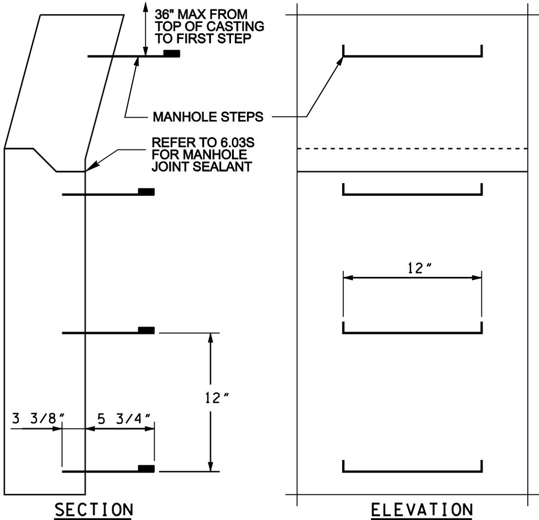
1. STEPS TO BE INTEGRALLY CAST INTO MANHOLE SECTION.
