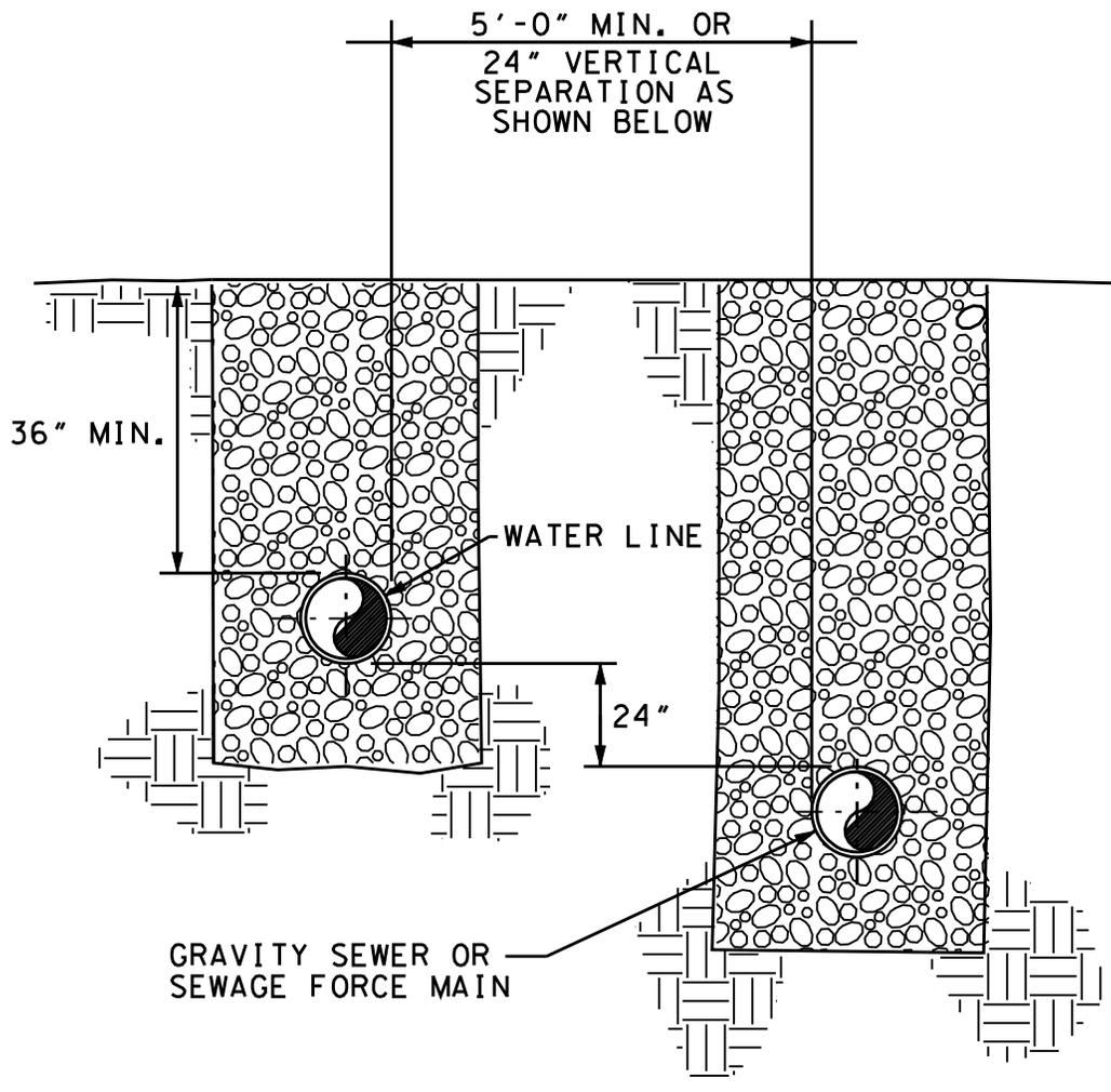
NOTE: IF SEPARATION CANNOT BE MAINTAINED, THE SEWER PIPE SHALL BE ENCASED A DISTANCE OF 5 FEET EITHER SIDE OF THE POINT OF CROSSING
