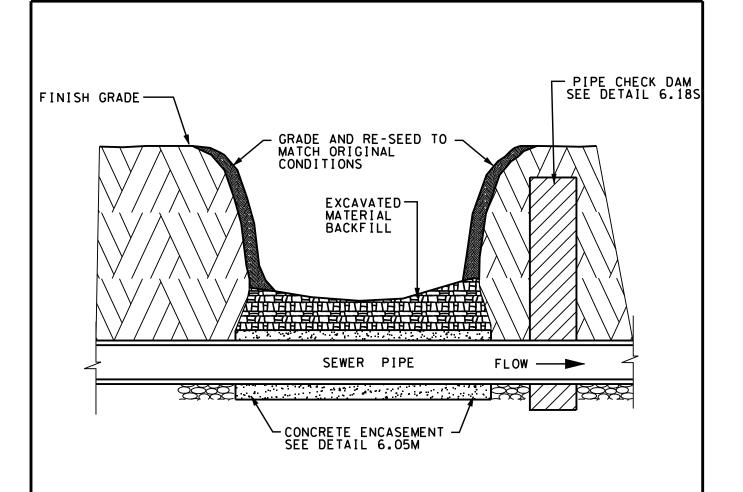
NOTE: FOR A NO-BLAST CREEK CROSSING, CROSSING IS TO BE PERFORMED AS FOLLOWS.
