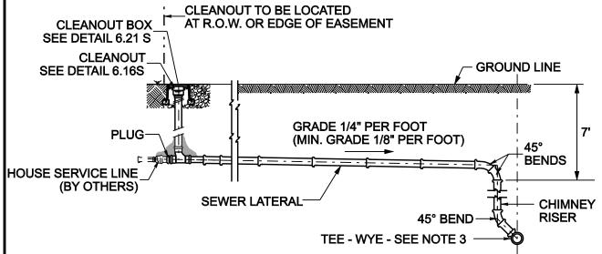
SERVICE MATERIAL TO BE SCH. 40 PVC. BACKFILL FOR SERVICE LINE TO BE SAME AS FOR SEWER LINE.
