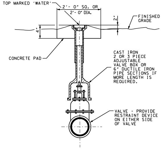
CAST AROUND THE TOP OF EACH VALVE BOX A CONCRETE DISK 2'-O" IN DIAMETER OR 2'-O" SOUARE AND 4" THICK WHEN VAVLES ARE LOCATED IN UNPAVED AREAS. NOT REQUIRED IN PAVED AREAS. PAD MAY BE PRECAST.
